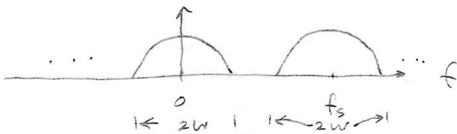
From the above diagram, it is clear that if the sampling frequency  $f_s$  is greater than  $2W$  Hz, the replica of the signal do not overlap with each other i.e., with no changes to the signal due to the sampling operations. Therefore, the original signal can be recovered by a low-pass filter.
