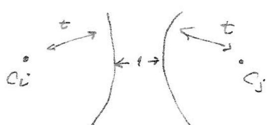
when there are at most  $t$  errors for both  $c_i$  and  $c_j$ , the resultant codewords still differ from each other by one Hamming distance. Therefore, the erroneous codewords can be corrected (or treated) as the "nearest" to the valid codewords.
