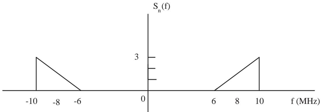
Figure 1.1 Power spectral density of  $n(t)$ .
